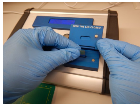
Figure 8. Inserting Gafchromic film into the DR4. The film should be handled with gloves or forceps.
