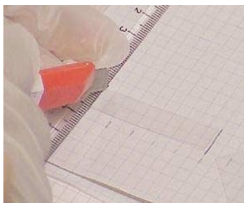
Figure 13. A sharp utility knife, a plastic ruler and a grid under the film help to cut it conveniently into desirable lengths.
