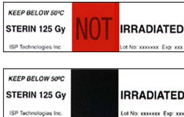
Figure 2.4: Radiation sensitive indicators before (top) and after (bottom) exposure at dose > 125 Gy (© ISP 2002).
