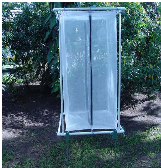
Figure 7.3: Field cage showing zippers on both sides as well as underneath the cage. Bottom opening used to introduce a potted plant. Side openings used for ease of access to collect dead sterile insects.
