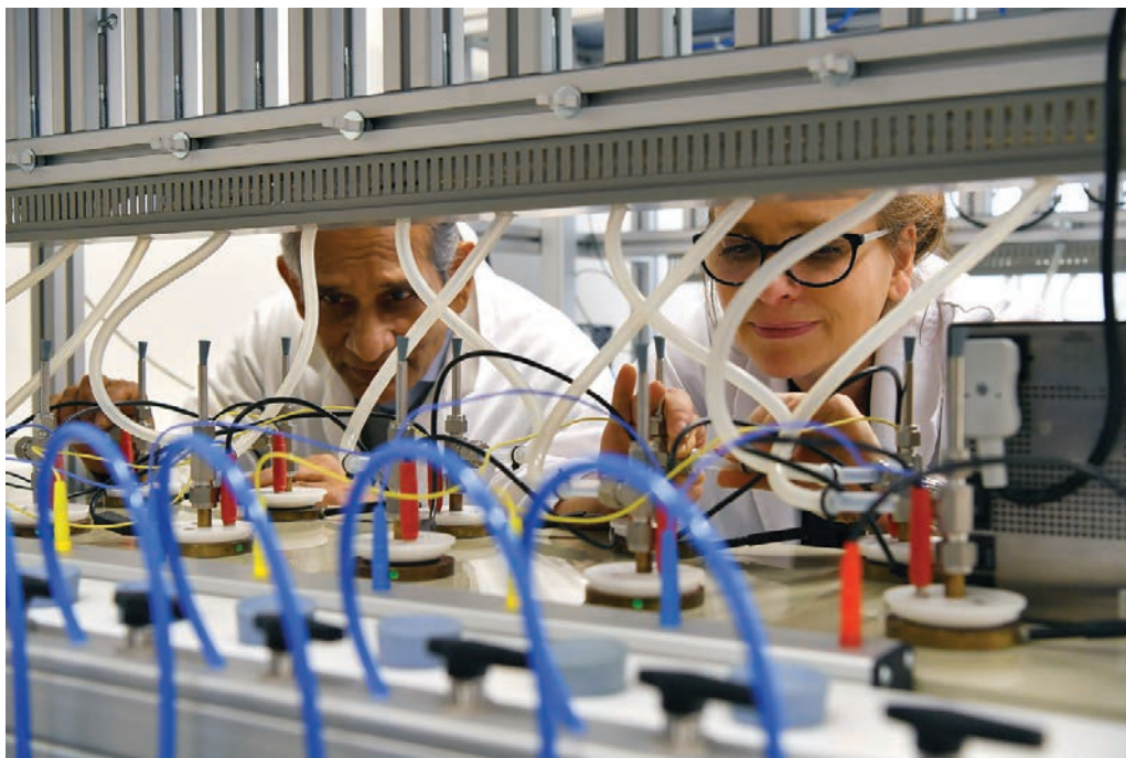
FIG. 2. Preparation of water samples for tritium analyses to be used for groundwater age dating purposes.
