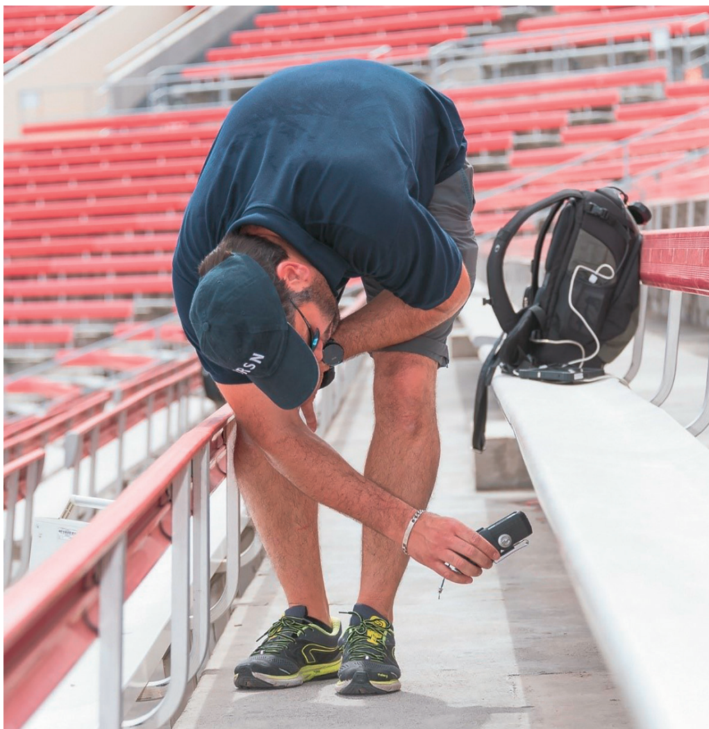
FIG. 1. A member of the RANET Joint Assistance Team ‘sweeps’ a stadium in Las Vegas (United States of America) to detect any hidden radioactive sources before a simulated major sport event. (Photograph courtesy of S. Carragher.)
