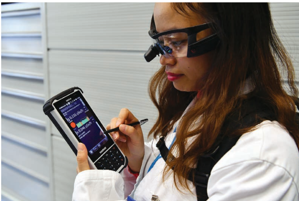
FIG. 4. An Agency safeguards inspector reviewing settings on a handheld unit of the Backpack Radiation Monitor, part of the Extended Multi-Component Inspector Kit (MCIK). The deployment of the MCIK was part of the Development and Implementation Support Programme for Nuclear Verification 2020–2021 (STR-393).
