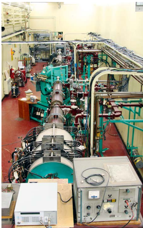
FIG. 1. A linear accelerator used for producing molybdenum-99 using the (\gamma, n) reaction on molybdenum-100. (Photograph courtesy of R. Galea, National Research Council Canada; Canadian Crown Copyright.)
