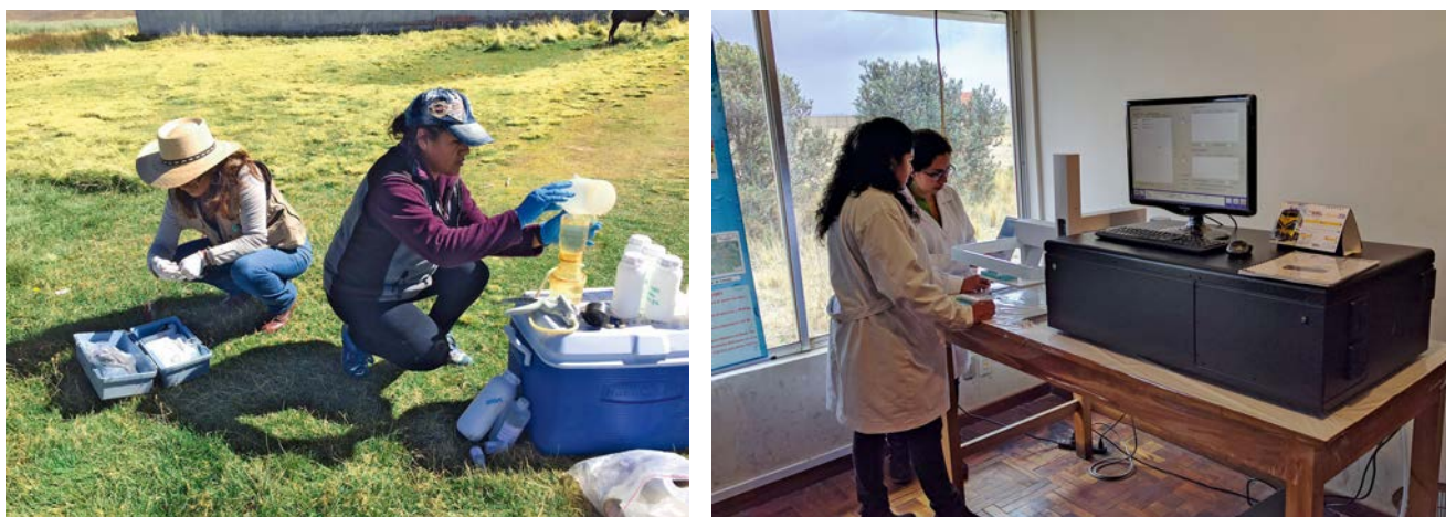
FIG. 1. As part of a technical cooperation project, Bolivian counterparts collect groundwater samples in the field (left), which are then analysed to measure the isotope ratios using a laser analyser provided by the Agency (right).
