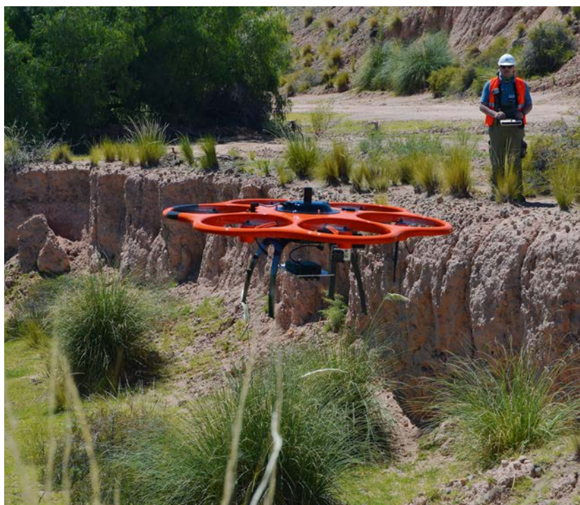
FIG. 2. As part of the Agency's unmanned aerial vehicle system for rapid environmental monitoring, drones mounted with sensors and cameras are used to remotely collect data in preparation for environmental remediation.
