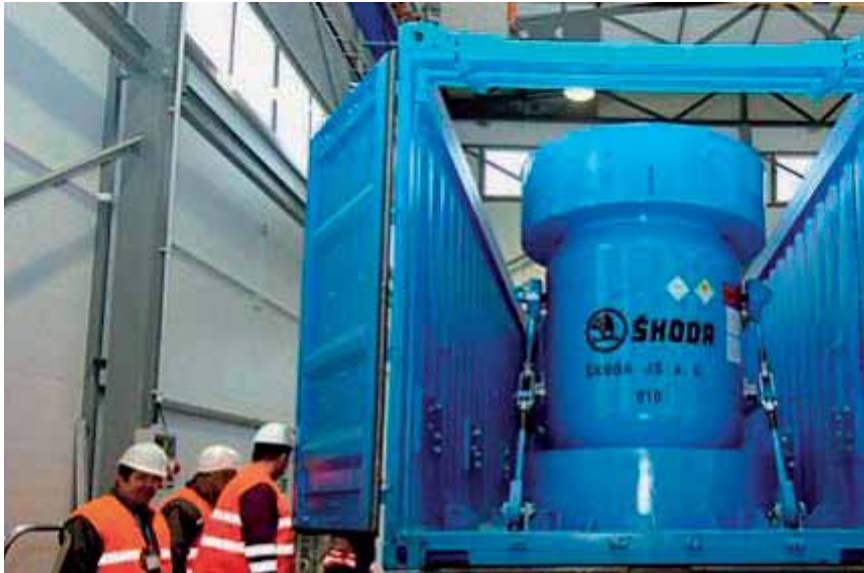
FIG. 2. High capacity cask used in the shipment of spent fuel from Řež, Czech Republic.
