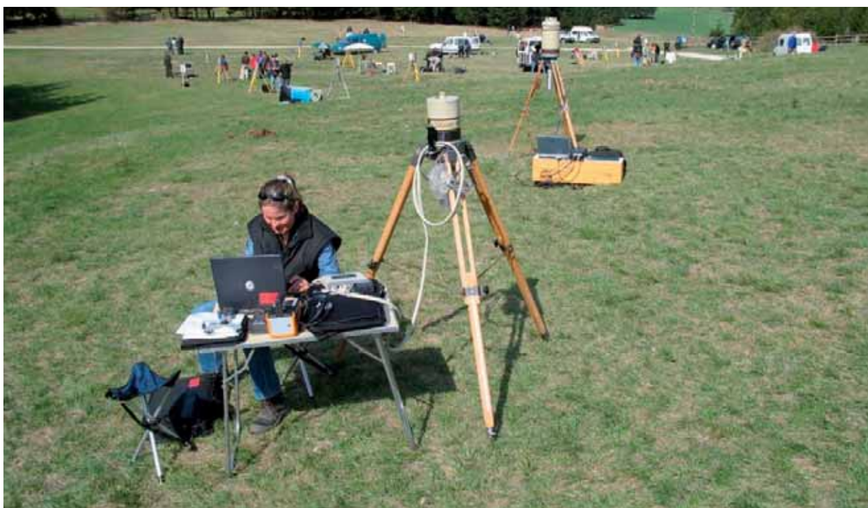
FIG. 2. High resolution gamma spectroscopy systems being tested under field conditions at the in situ intercomparison scenario exercise in Austria.
