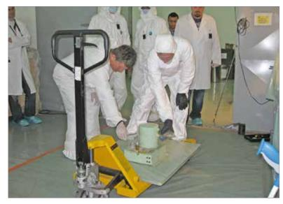
On the second day of the training participants were able to observe a real-life conditioning operation at Montenegro's national radioactive waste storage facility. Devices containing disused sealed radioactive sources, collected from all over the country, are stored here awaiting further management.
