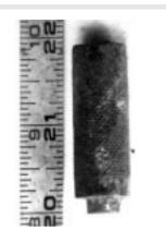
An unshielded caesium-137 found buried in gravel at a metal scrapyard in Illinois. The scale is in inches.
