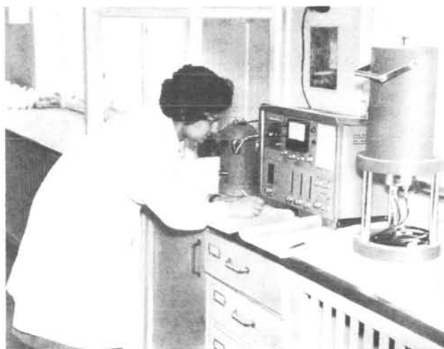
An assistant at the laboratory reads from a scaler the radioactivity of samples contained in one of the adjoining detecting instruments
