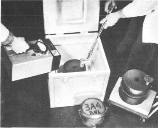
Safety regulations in operation in the USA. Photo shows a radioactive sample, ready for shipment, being put in a lead shield centered in a wooden box for radiation protection required by regulations of the Interstate Commerce Commission. A radiation meter is being used as a safety precaution for personnel
