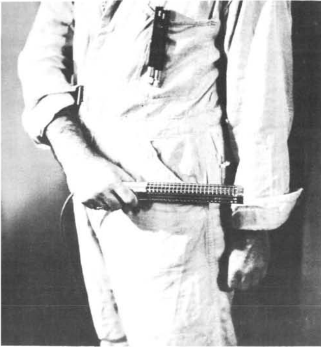
A handy instrument for a radiation worker to monitor all parts of his body and clothing
