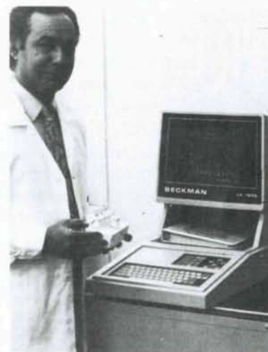
At the chemistry unit, a liquid scintillation counter for strontium-90 and tritium.
