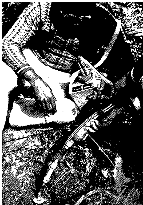
Figure 5. Measurement of radon gas in soil.
