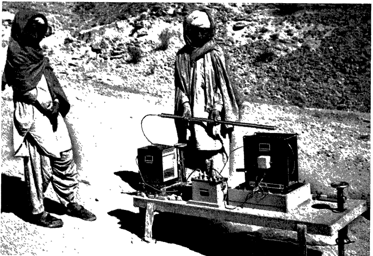
Figure 3. Borehole logging in Pakistan. The worker is standing behind the logger recording apparatus and the manual winch used to lower the probe into the hole, and is holding the probe itself in his hands.
