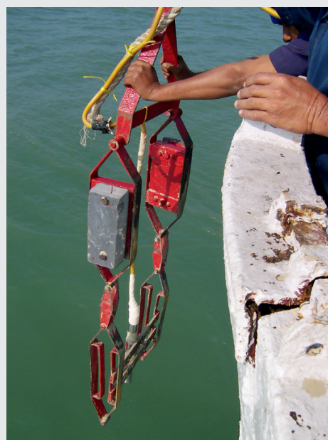
Post-injection monitoring of a radiotracer as part of sediment transport investigation conducted at the Kolkata Port, India, in 2016.
