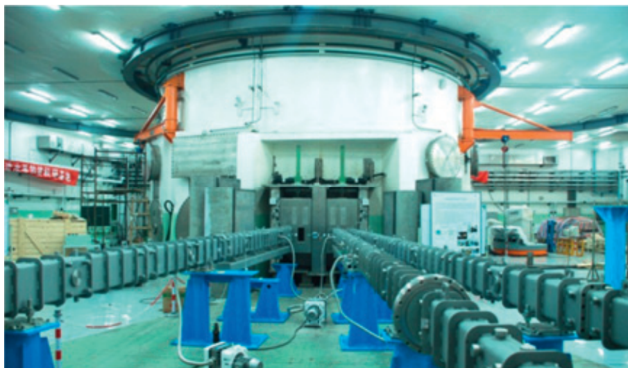
FIG. 2. Hall of small angle neutron scattering beam lines of CARR (source: CIAE).
