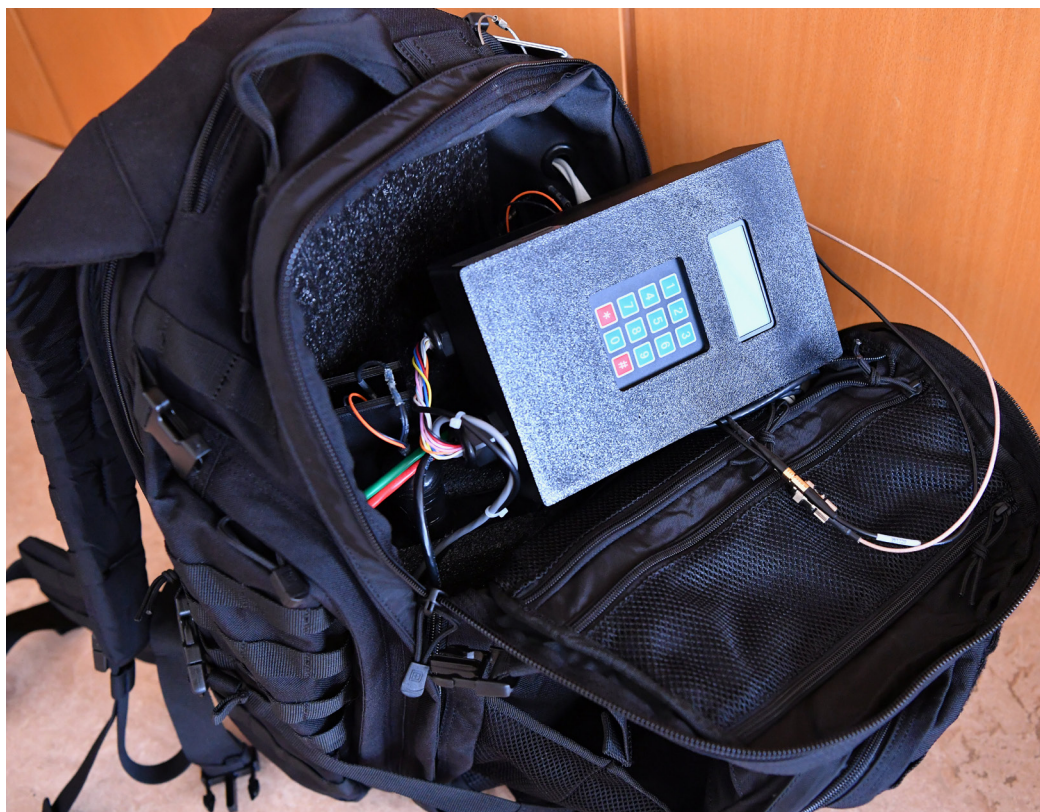
A look inside a radiation detection backpack.
