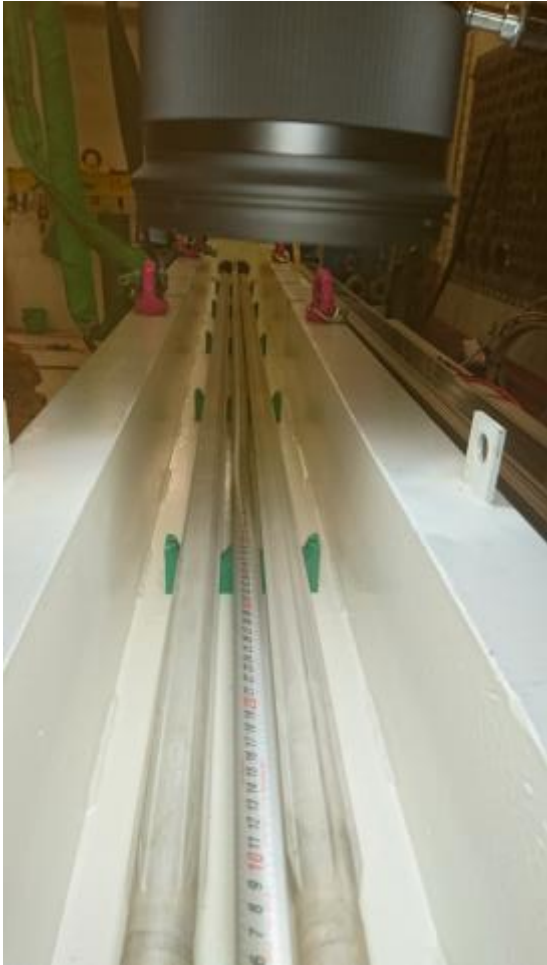
Figure G-2: The visual inspection equipment for the historical spent fuel at HBWR
