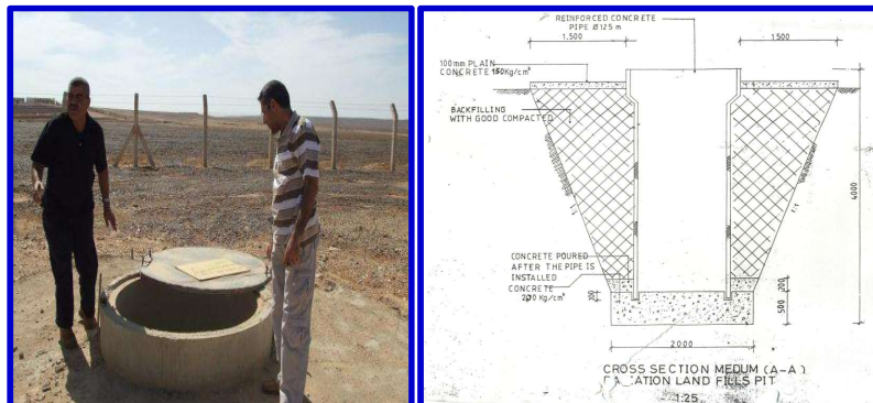
Figure L.9 Left: The cylindrical underground reinforced concrete pit; , Right: The layout diagram of the cylindrical underground pit
