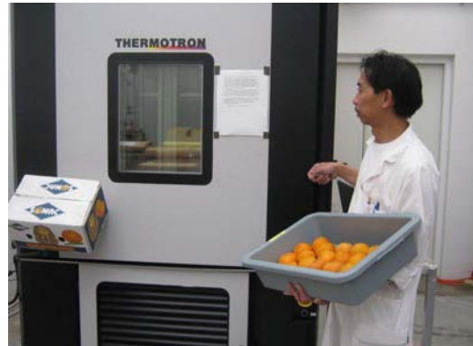
FIG. 9. Environmental chamber used for the cold treatment of Bactrocera zonata .
