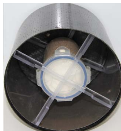
FIG. 1. PBGL scientists have developed a range of specialized adaptors for irradiation of seed and tissue culture materials using X ray equipment employing orbital rotation around an X ray source.
