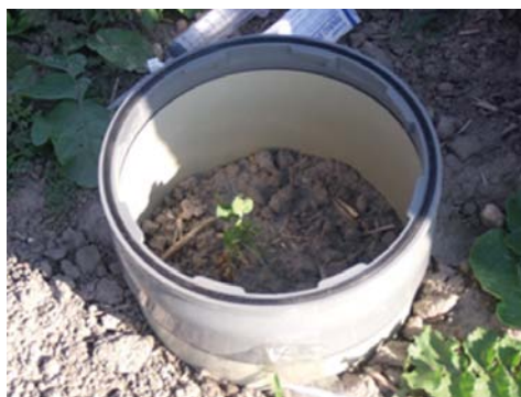
FIG. 1. Low cost gas chamber for measuring nitrous oxide gas.
