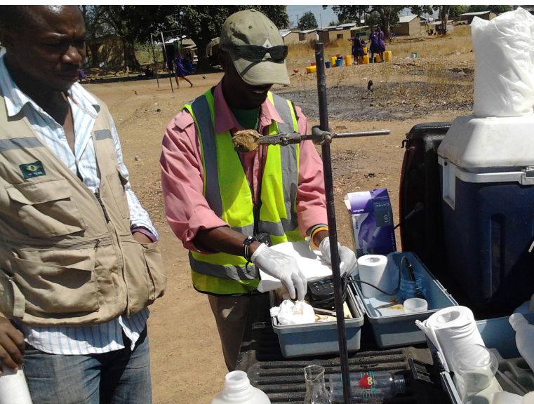
Sample preparation for tritium analysis of groundwater, Isotope Hydrology Laboratory, Ghana Atomic Commission.
