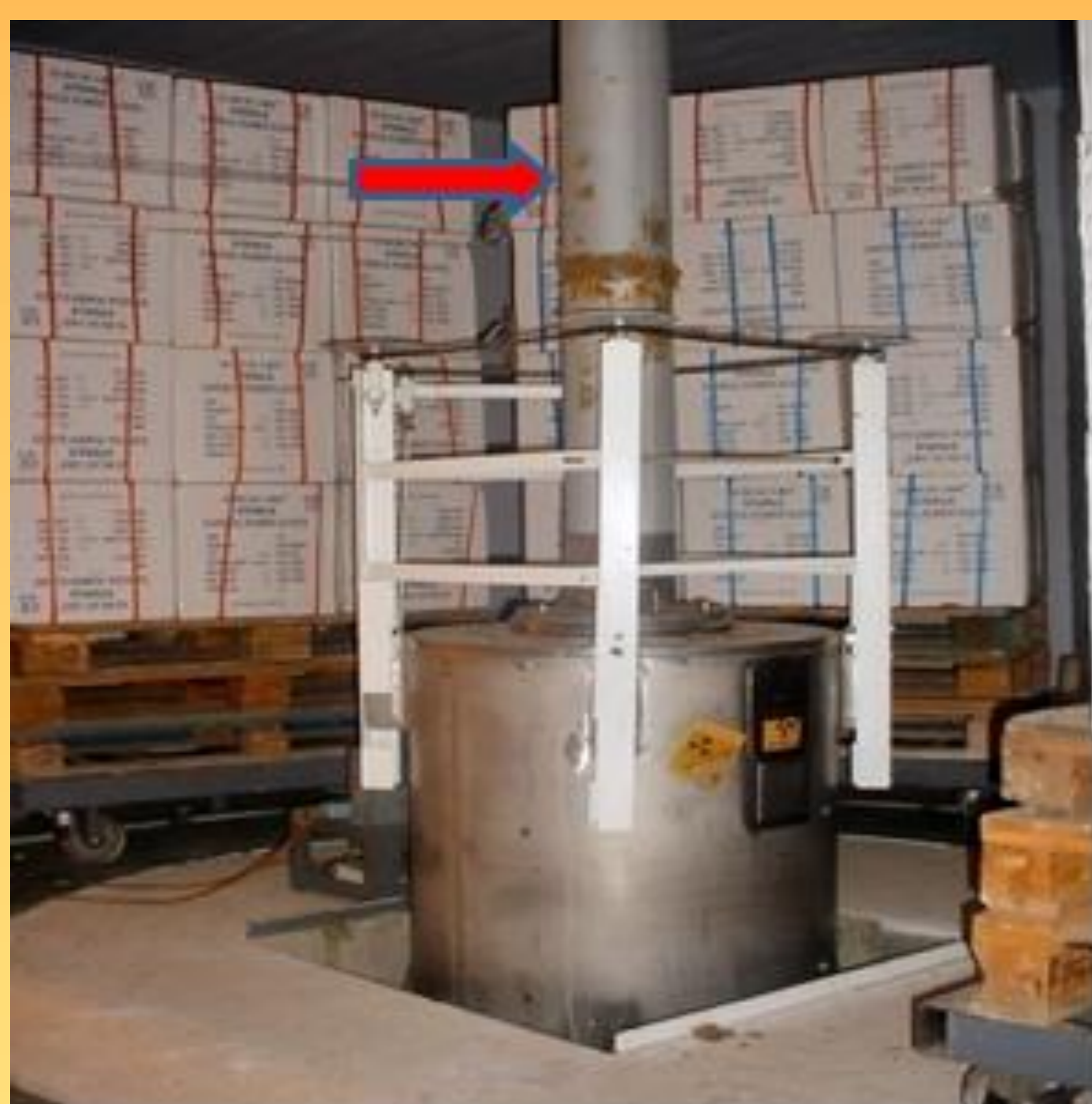
Fig. 2. Indication of the irradiation position in the source building : the rate dose is measured to 47.62 Gy/min.
