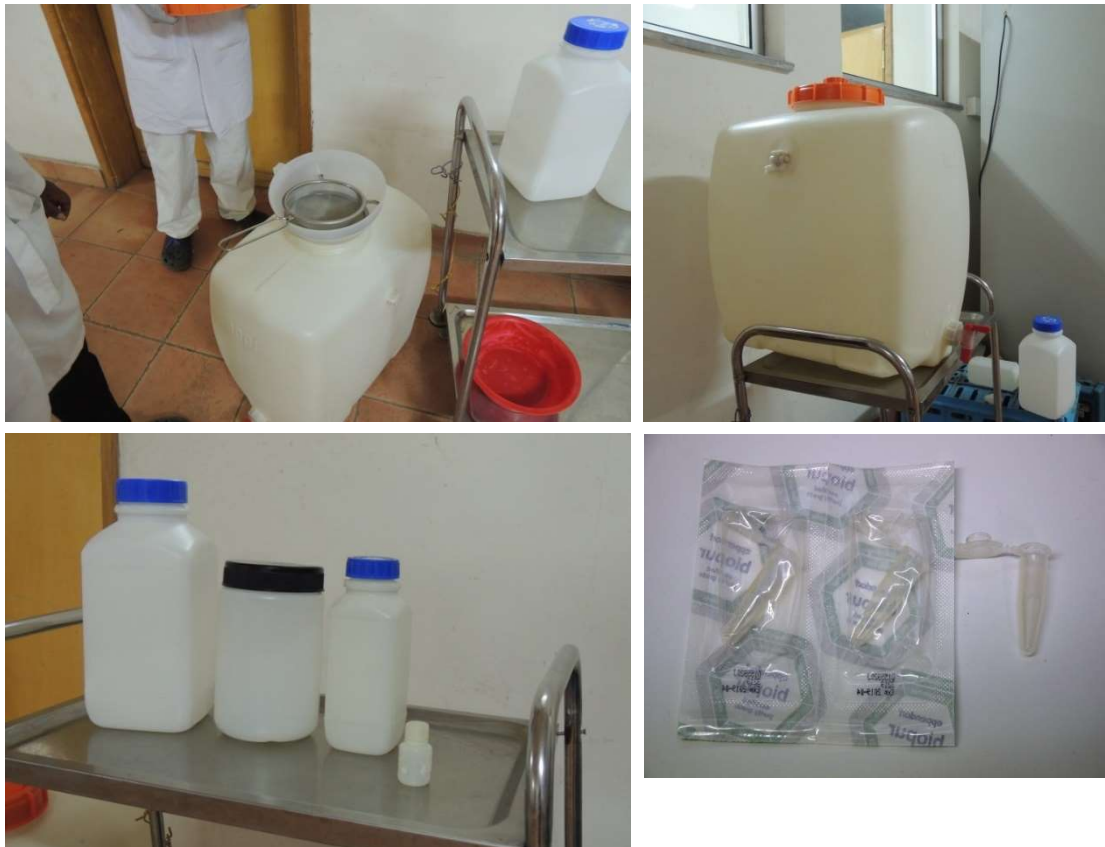
Figure 5. Some of the blood proportion equipment (funnel, sieve, 100L container, storage bottles of 4L, 2L and 1L capacity, Eppendorf tubes).
