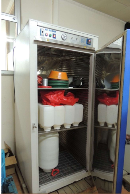
Figure 2. Heat sterilization of blood collection equipment in oven.
