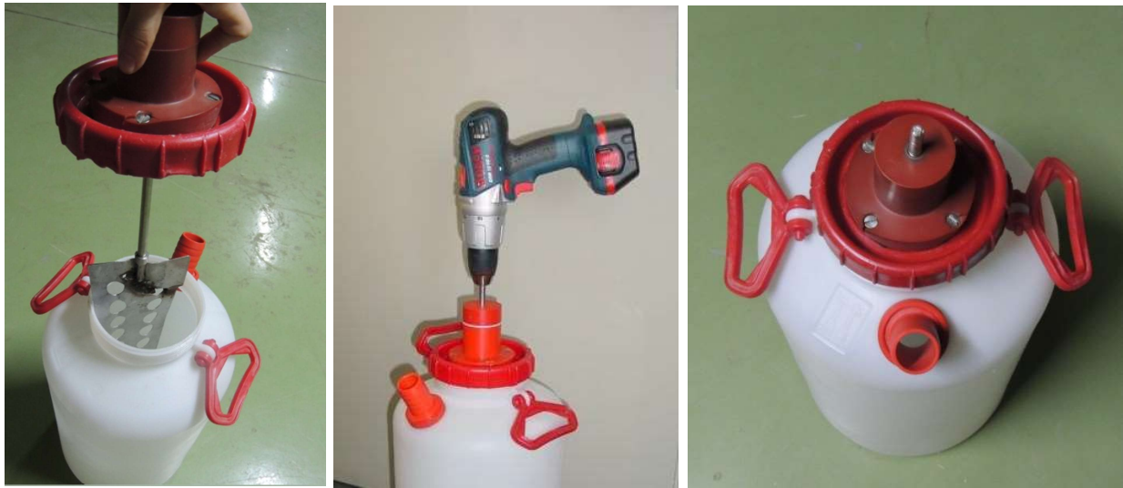
Figure 3. Defibrination set (mechanical handheld drill and paddle), 25-litre container with side inlet.
