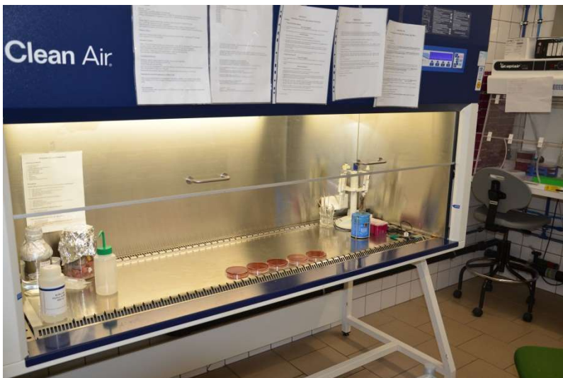
Figure 9. Laminar flow bench with the equipment used for the microbial screening.
