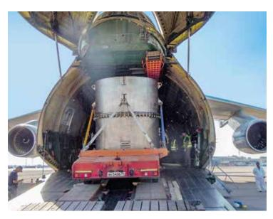
FIG. 2. A truck carrying a transport canister with irradiated liquid HEU fuel drives into a cargo plane for repatriation of the fuel to the Russian Federation.
