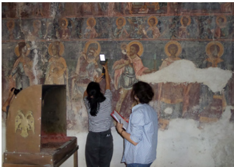
Applying nuclear techniques to characterize cultural heritage artefacts in Albania. (Photo: Institute of Applied Nuclear Physics/ Albania)
