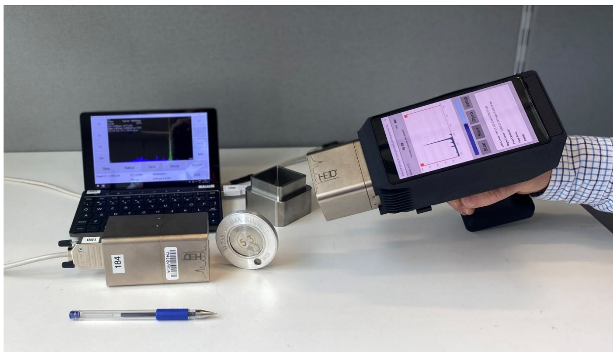
The next generation of IAEA gamma spectrometry instruments: MCCM (left) and HM6- (right) (Photo: IAEA)
