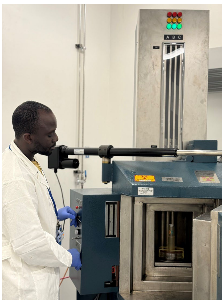
FIG. B.1. A PhD student from Burkina Faso setting up the model 812 irradiator to expose the tsetse pupae. (Source: IAEA)
