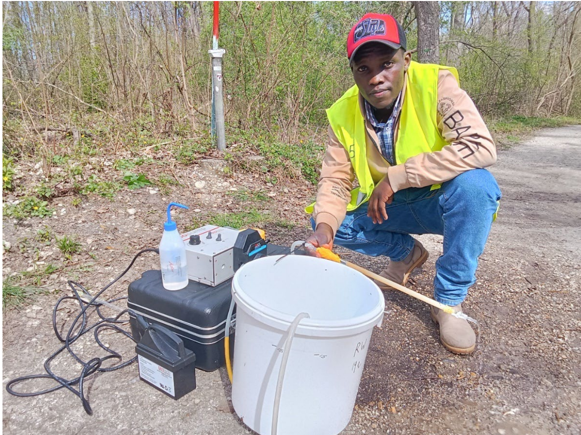
FIG. B.1. Testing the collection of water samples for analysis of sulphur-35 to determine short residence times in groundwater. (Source: IAEA)
