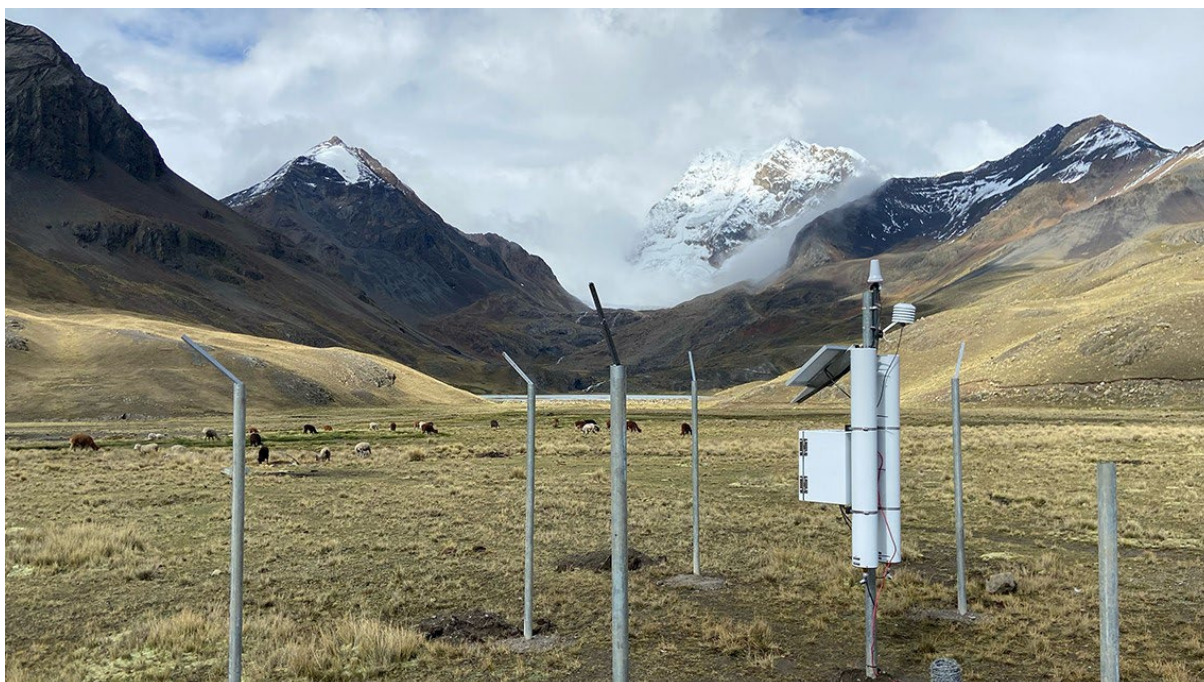
FIG. B.3. A cosmic ray neutron sensor installed in high Andean Bolivian wetlands to study their role in buffering water in the context of climate change. (Source: Trenton Franz)
