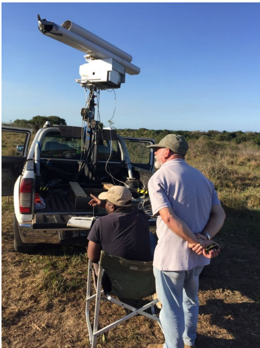
FIG. B.6. The harmonic radar system used in Mozambique to track individual tsetse flight. (Source: IAEA)
