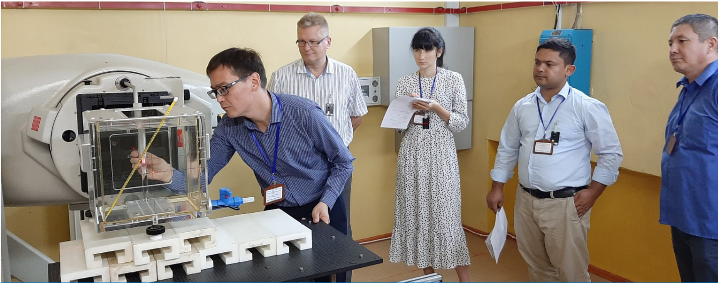
Positioning an ionization chamber during a practical session organized through KAZ6012. (Photo: N. Mamyrbek)
