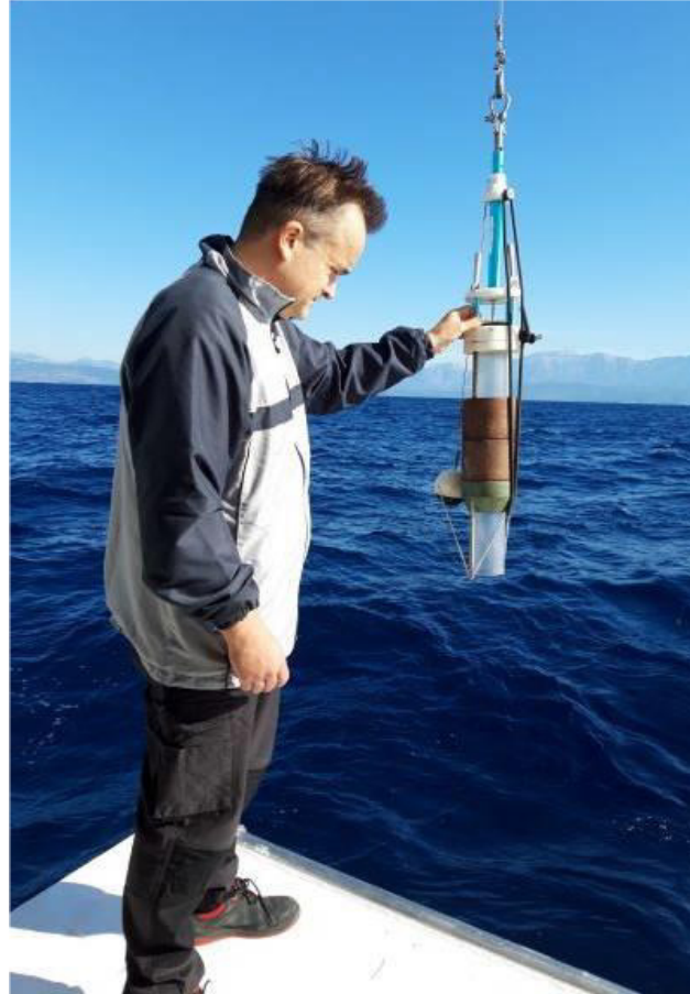
Sediment core taken from the Mediterranean coast during the sampling expedition organized within a project workshop that took place in Kotor, Montenegro, October 2019. (Photo: J. Obhodas/ Ruđer Bošković Institute)
