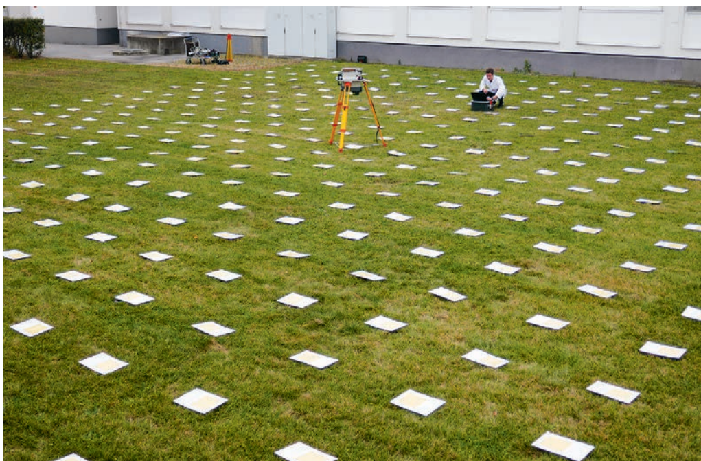
FIG. 1. Field calibration of gamma spectrometers using a novel technique of imprinting paper sheets with radionuclides; the technique, developed at the Agency, is now also used for proficiency testing.
