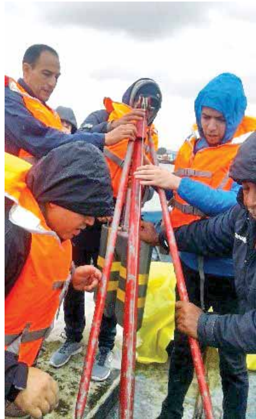
Participants preparing the nucleonic gauge for sedimentation measurement. Photo: Reinhardt Pinzon/UTP
