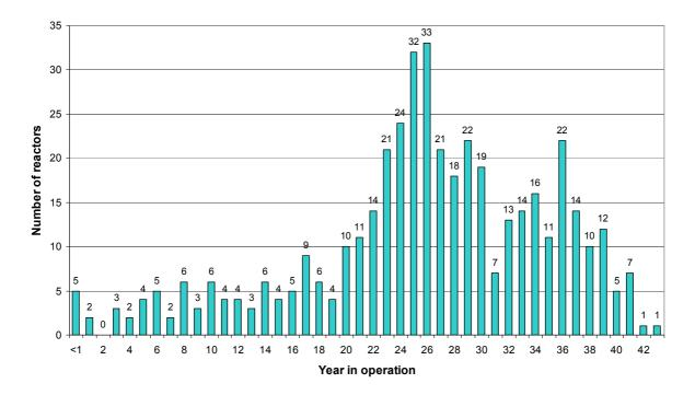
FIG. B-3. Number of operating nuclear power plants by age in the world as 26 August 2010 (note that a reactor's age is determined by the date when it was first connected to the grid)
