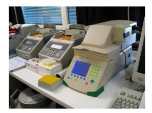
FIG. II-3. Different models of thermal DNA amplification cyclers (PCR Machines). Isothermal DNA amplification technologies will reduce our reliance on this expensive equipment.
