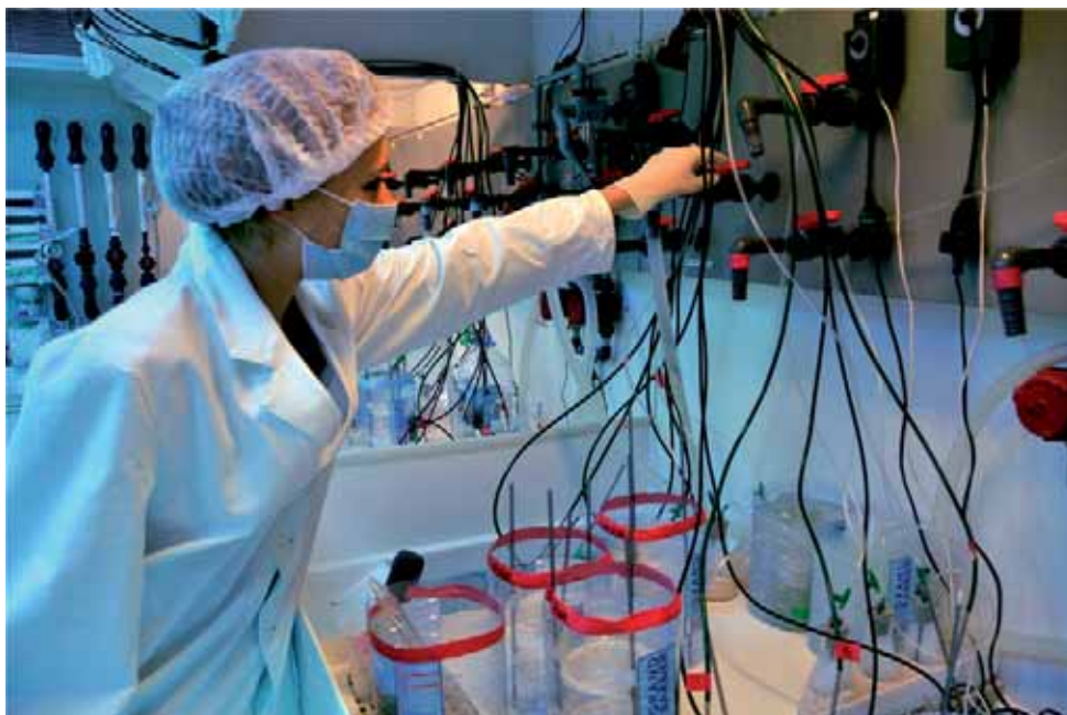
FIG. 1. An experimental system at IAEA-MEL to assess the impact of exposure of commercial seafood to seawater at the decreased pH levels predicted by climate change models.
