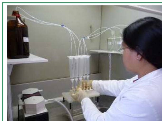
Figure 4. Extraction/concentration of water samples on SPE cartridges.
