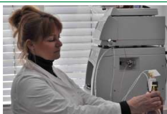
HPLC method developed by Strathclyde University and the Agrochemicals Unit for the quality control of isometamidium products.
