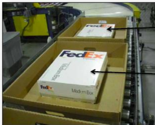
Fig. 7: Prototype single and double stacked guava packages on E-beam processing conveyor belt.
