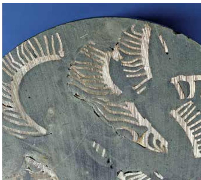
Cement-encapsulated Magnox fuel-cladding at Sellafield (Photo: Sellafield Ltd., UK)
