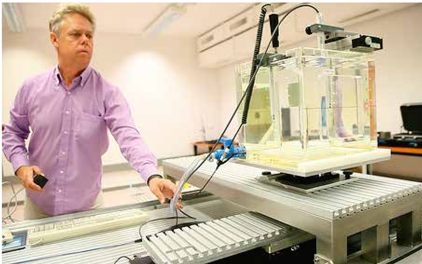
Setting up equipment for dosimetry calibration at the IAEA Dosimetry Laboratory (Photo: Rodolfo Quevenco, IAEA)
