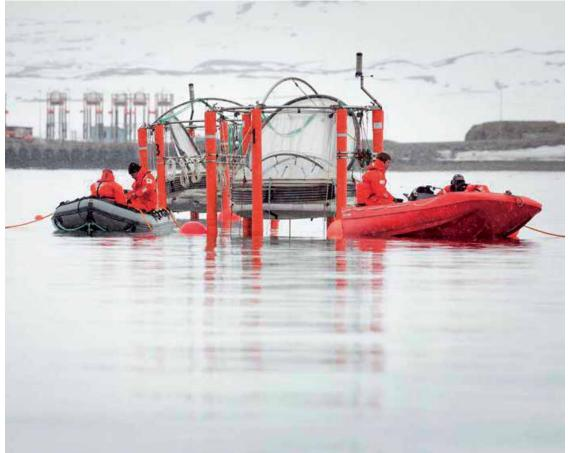
Radiotracer studies can be applied in floating or seabed tent structures called mesocosms. This valuable experimental tool allows natural environments to be studied under controlled conditions combining the benefits of lab and field work. (Photo: Nick Cobbing)
