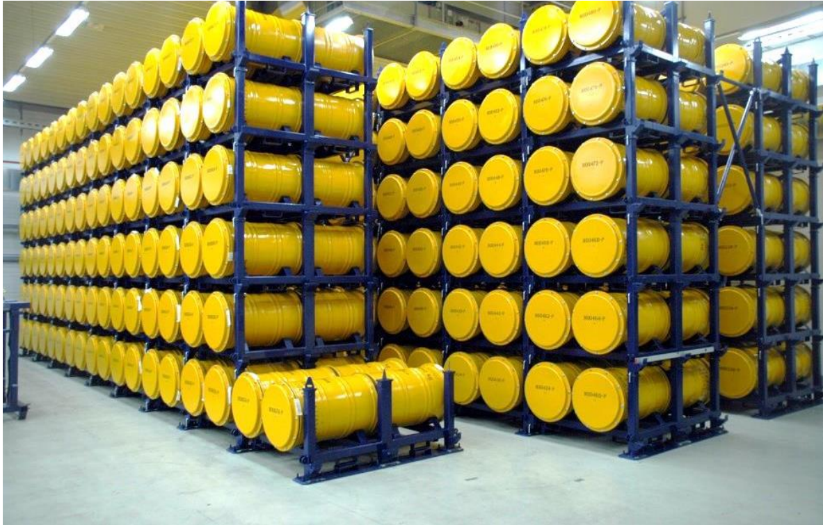
Figure 5 Conditioned waste in interim storage facility 13, © NES
