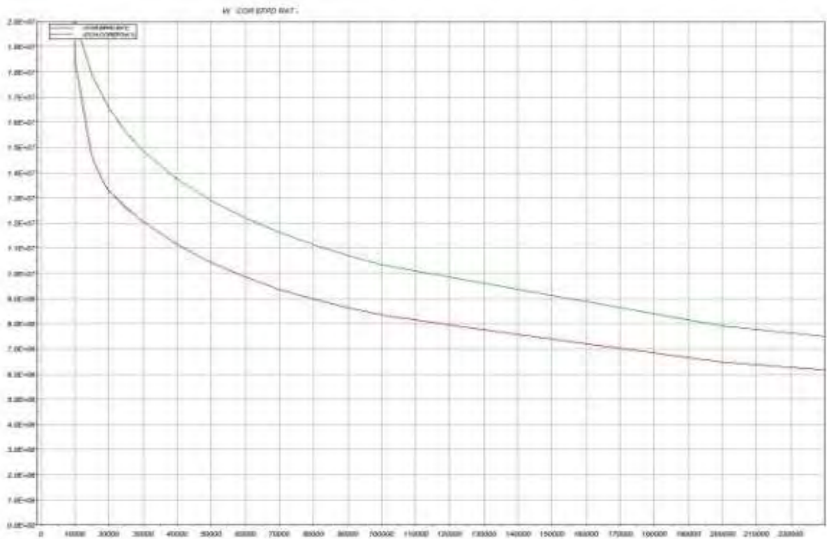
Figure N° 3-28: Total and actual core power [MW], time in[s], case with open cavity connection & increased water amount
