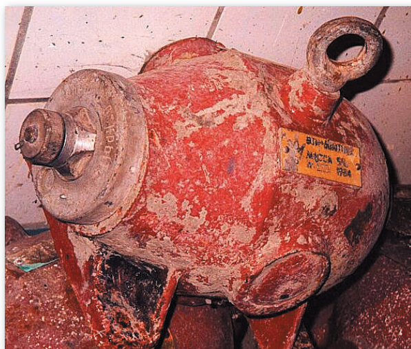
FIG. 2. Disused radioactive source (level gauge with caesium-137).
