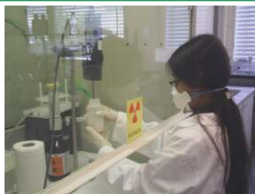
Preliminary optimization of the extraction step using 14 C labeled pesticides.
