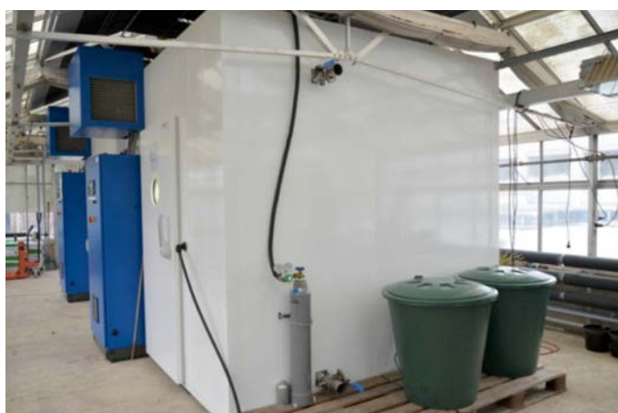
FIG. 6. Walk-in growth chambers with adapted CO 2 regulation and automatic irrigation system
