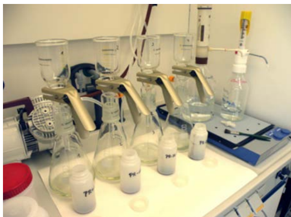
FIG. 8: Filtration of the HCl-extract of different phosphate rock samples
