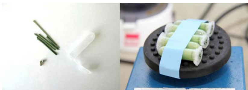
Leaf tissue dried using silica gel (left) is easily ground using metal beads and a standard vortex mixer found in most laboratories.
