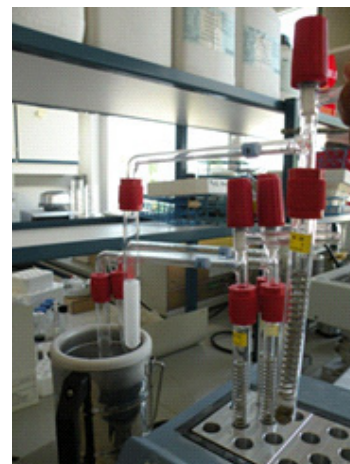
FIG. 7. The vacuum distillation system for extracting water from soil and plant samples for oxygen isotope and deuterium measurements.
