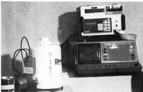
System for plutonium isotopic analysis with multichannel analyser and detector
