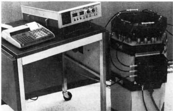
System for plutonium isotopic analysis with multichannel analyser and detector
