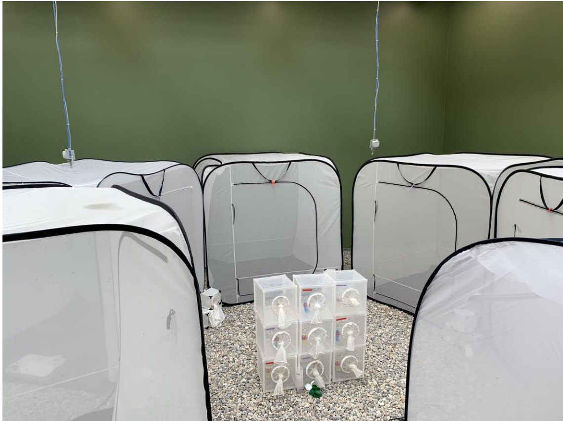
Figure 2B. Example of a semi-field cage experiment setting: Nine 30×30×30cm control cages (irradiated (low, high doses) and non-irradiated males only) and six large competition cages, each containing 100 males (irradiated and/or non-irradiated) and 100 virgin females. Low and high stand for low irradiation (inducing more than 99% sterility) and high irradiation dose (100Gy more than the low dose)
