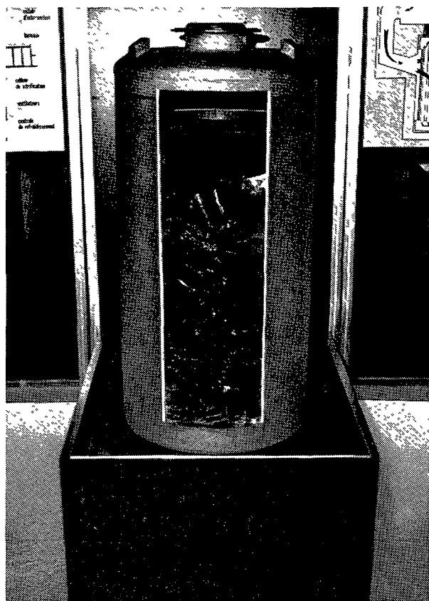
Model of a prototype container of vitrified nuclear waste, showing the borosilicate glass inside.
