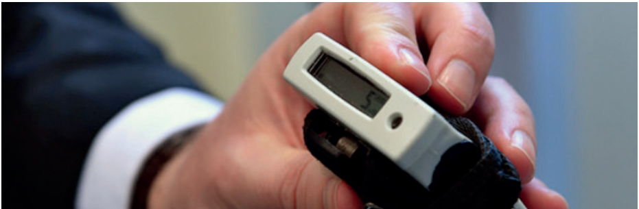
An electronic personal dosimeter worn by workers who might be exposed to radiation.
