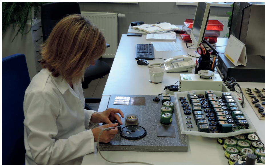
Preparation of radon dosimeters that will be used by workers who might be exposed.
