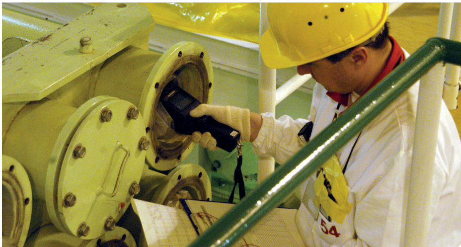
A worker checks the radioactive contamination level on the inner surfaces of a pipe.
