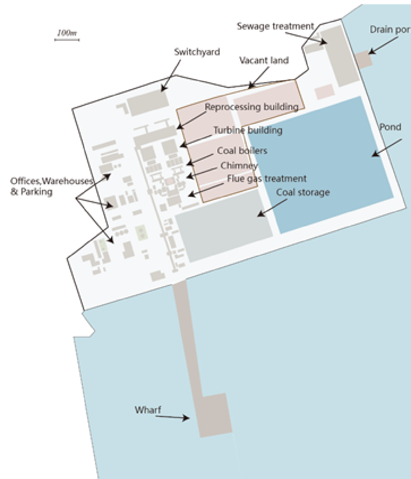
Fig. 11 Repowering a large coal-fired power plant with 2 \times 600 MWe HTR-PM modules.
