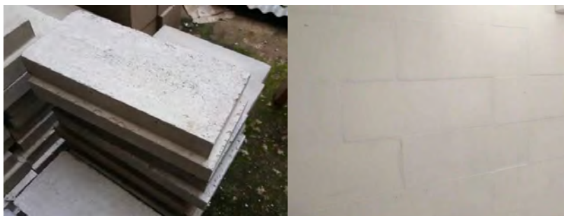
FIG. 15. Concrete blocks for 'sacrificial' layer
