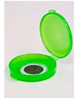
FIG. 3. Exposed stretched Teflon filter, optimised for IBA analysis.
