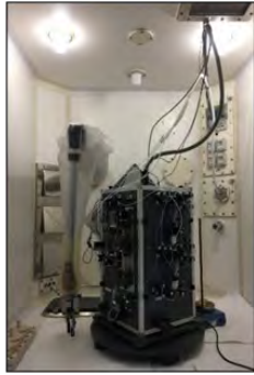
FIG. 16. Thallium Chemistry hotcell with Tl-chemistry module
