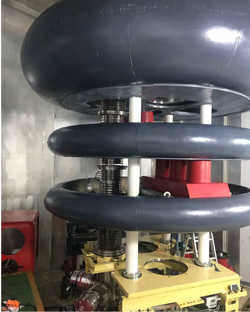
FIG. 2. Single-ended, modular ESQ accelerator. Operates in air for easy maintenance. This machine has 720 kV. The full size one of 1.45 MV is being constructed. Reprinted from Ref. [27]
