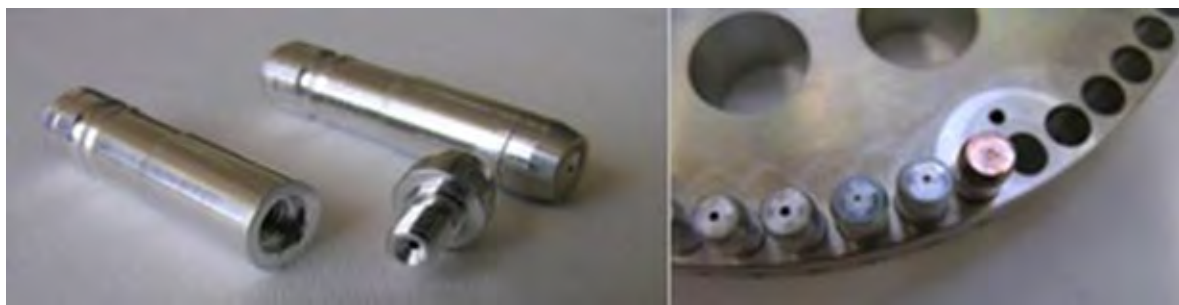
FIG. 10. Typical cathode systems used in the accelerator ion source for AMS studies, left is a cathode and right are cathodes in an ion source cathode wheel.
