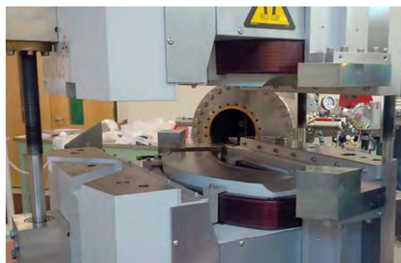
Figure 4: High Energy Permanent Magnet with upper yoke lifted during assembly. Note the small size of the trim coil compared with the space available for a water-cooled full power coil.
