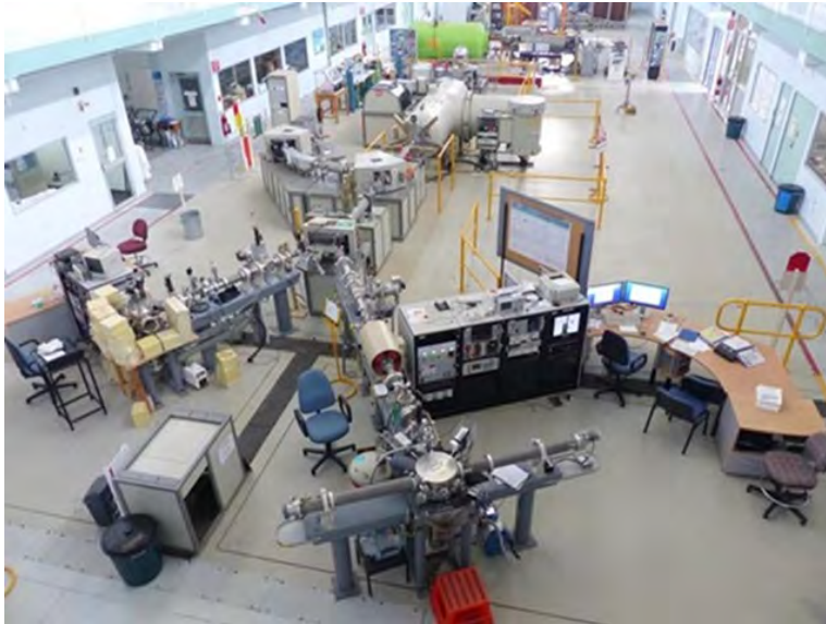
FIG.2. ANSTO 2MV STAR accelerator used in IBA studies
