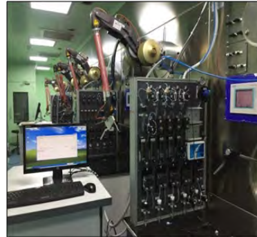
FIG. 17. Thallium Chemistry External Panel: computer-based controller system
