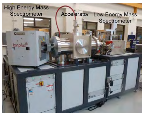
Figure 3: Single Element ^{14}\text{C} System installed at Lalonde AMS
