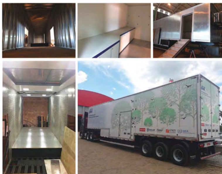
FIG.4: Mobile electron beam irradiation unit for the treatment of industrial effluents in Brazil.
