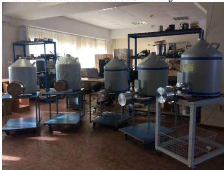
FIG. 4. BSI production of large diameter HPGe detectors for gold analysis.
