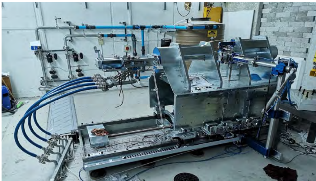
FIG. 8: The prototype target station being commissioned.
