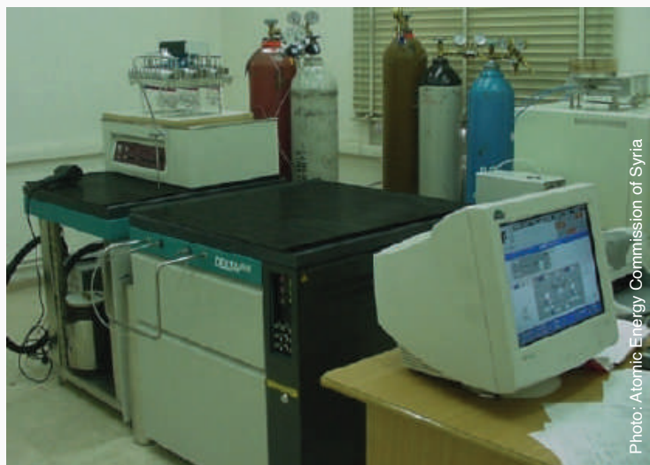
▲ Facilities for stable isotope analyses in water samples at AECS (Syria): Finnigan MAT DELTAplus mass spectrometer
