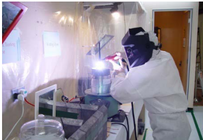
Source Containment (welding)
